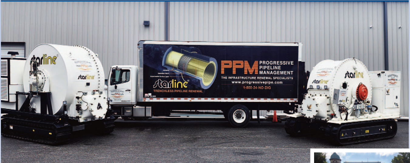
Two of PPM's six Starline® cured-in-place-lining inversion drums for lining mains from 12 - 48 inches. "Kong" is on the left and "King Ghidorah" on the right.
