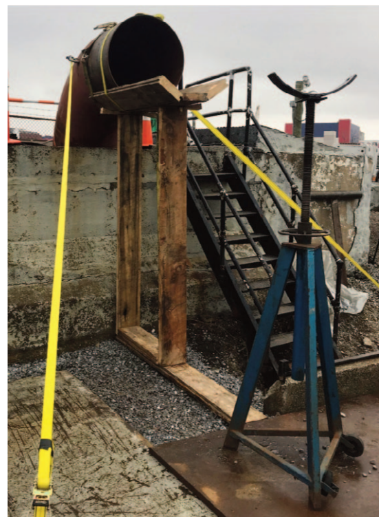
The "change in direction" fitting redesigned the profile from a vertical downward connection to a horizontal connection
