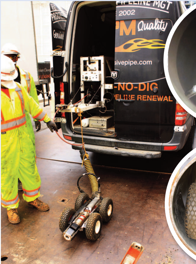
ARIES LETS CCTV robotic camera inspects mainlines and laterals prior to and after lining.
