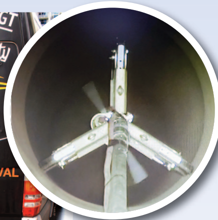
The 30-inch spin blaster is used for sandblasting. It can clean mains from 16 - 48 inches.
